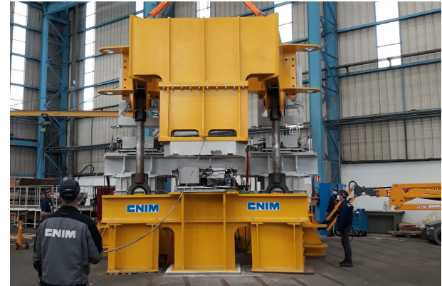
Testing one of the tools for mounting components for the ITER fusion reactor.
