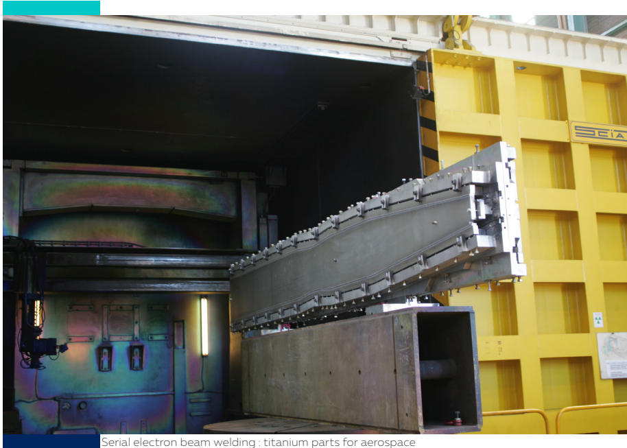
Serial electron beam welding : titanium parts for aerospace
