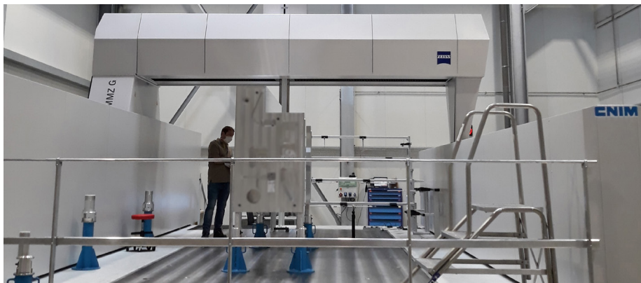
Check to the nearest tenth of a millimeter with the ZEISS MMZ-G machine. (X 4000 Y 8000 Z 2000 mm)
